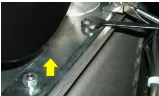
- Remove the screws "B" (with 13 mm socket wrench / 13 mm hex spanner) and remove the fastening plates
